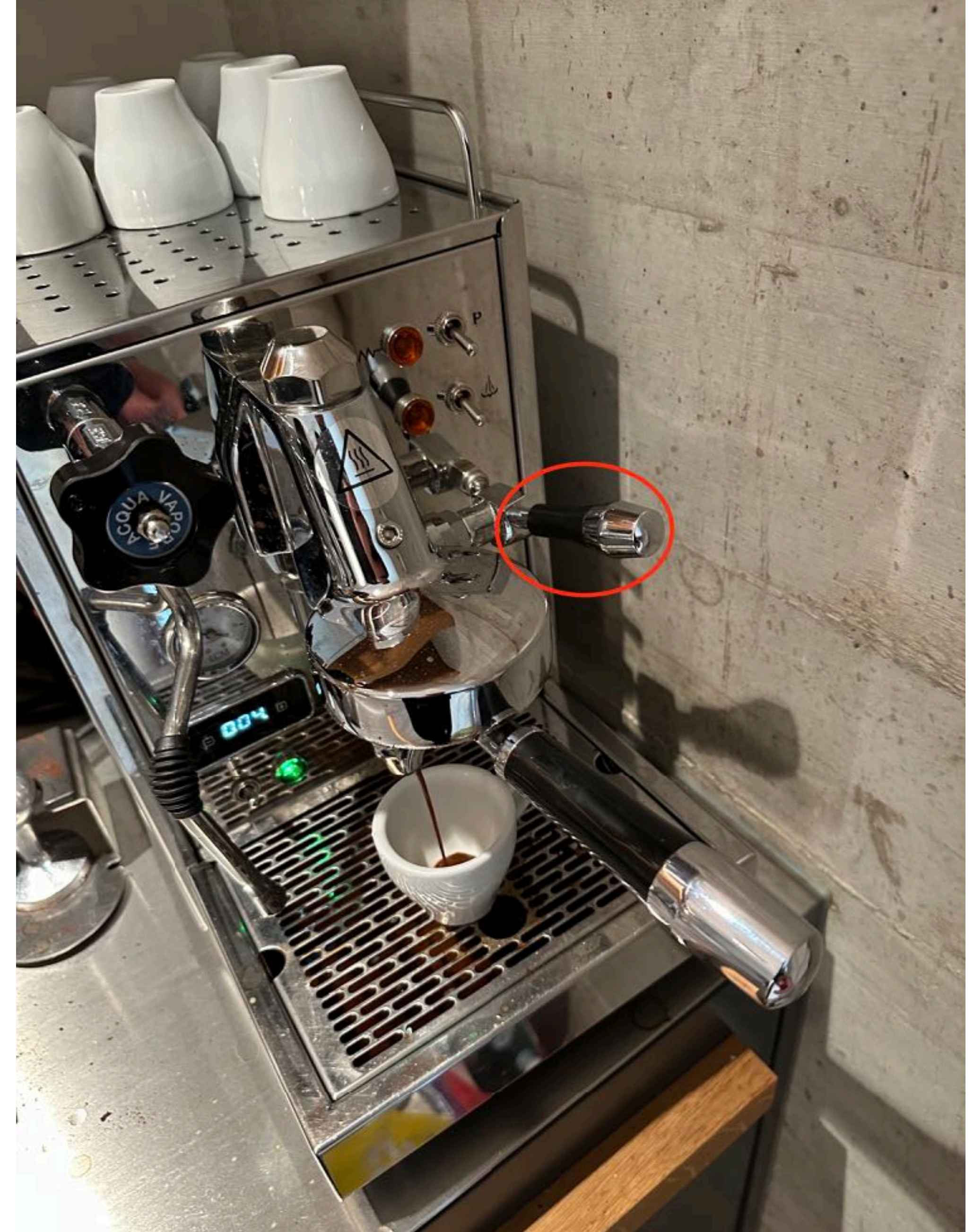
3) PULL LEVER UNTIL FILLED, THEN PUSH DOWN
